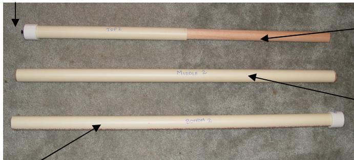
**Top pole** – 1/2 length PVC, full length dowel. Glue dowel, PVC and end cap together.
